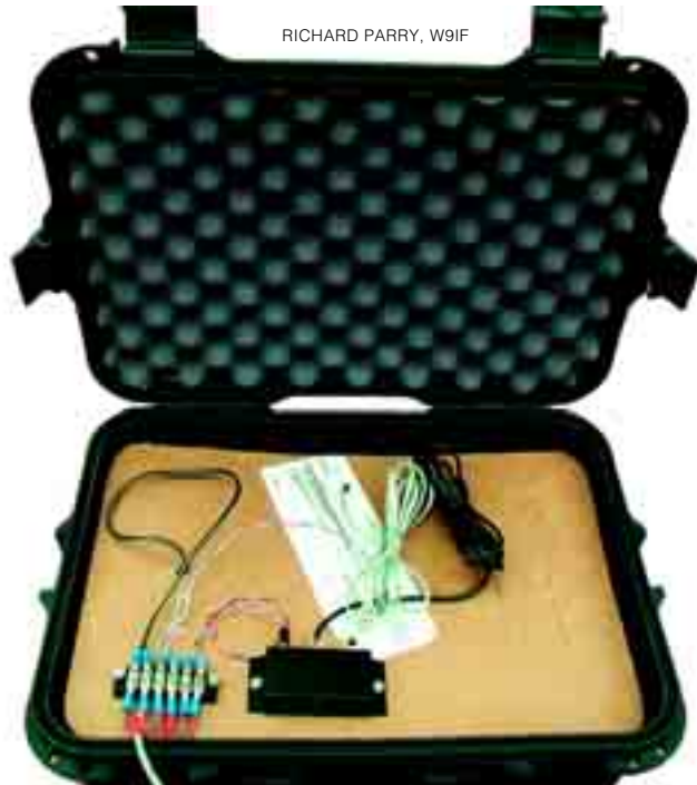
Figure 3—Bottom view of the APRS weather station. The terminal block provides for power distribution, while the junction box in bottom center interfaces the outdoor temperature sensor and anemometer.
