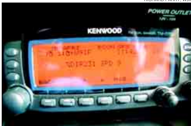
Figure 5—A Kenwood TM-D700A with voice synthesizer provides both visual and aural notification of weather conditions. The D700A speaks wind speed and direction without requiring driver visual interaction.
