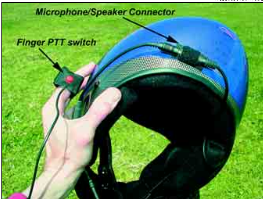
Figure 8—A view of the finger PTT switch and connector that interfaces the speaker and microphone inside the helmet.
