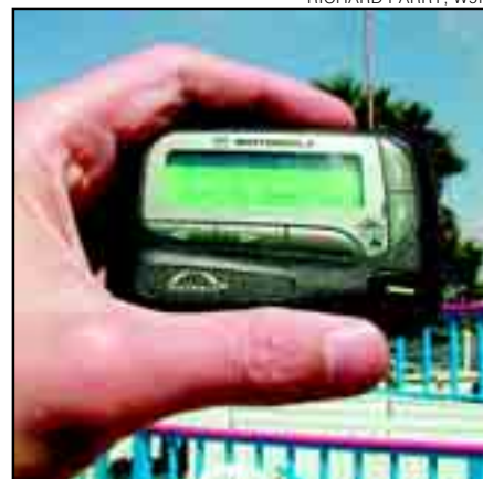
Figure 6—A commercial pager can be used to display weather conditions. Here, the display shows that the wind is from the SSW (216°) at 14 mph.
