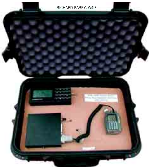
Figure 2—Top view of the weather station in its weatherproof enclosure. The Ultimeter 2000 (Peet Brothers) is in the upper left and a Kantronics KPC-3 Plus TNC is in the lower left. An ICOM IC-W21AT on the right is used for communication.
